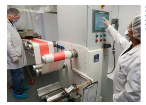
Figure 1: The film and liner exit the oven and are stored as master rolls, ready to be divided into daughter rolls and further into single doses.
