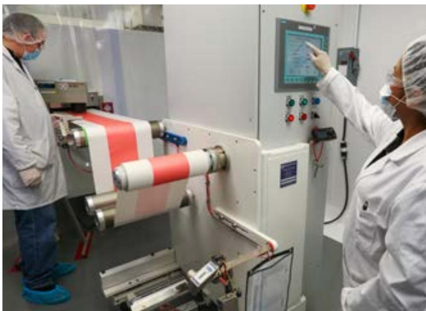
Figure 1: The film and liner exit the oven and are stored as master rolls, ready to be divided into daughter rolls and further into single doses.
